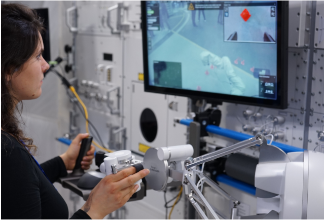
Figure 13: Operator controlling the rover with sigma.7 during the preliminary user test.
